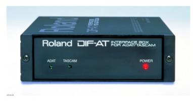
The Interface box for ADAT/Tascam converts signals between RMDB2 and ADAT/Tascam T/DIF and handles 8-in/8-out digital audio. It is 1/3 rackmount size.
